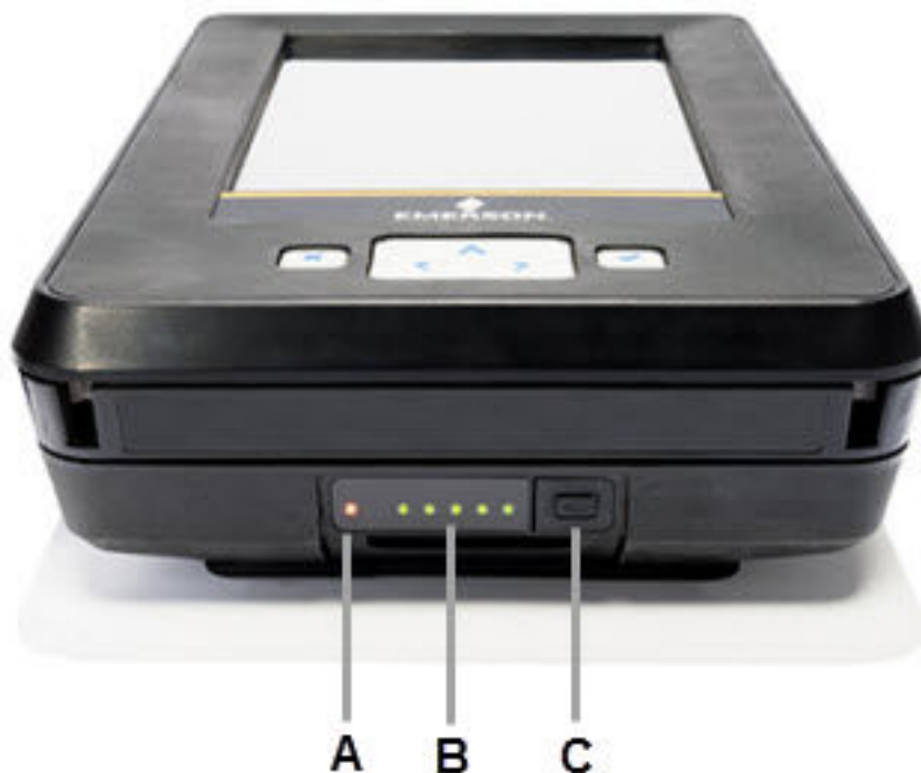
Figure 2-9: LEDs showing approximately 100 percent charge
