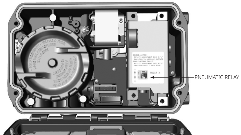
Figure 20. Pneumatic Relay Location
